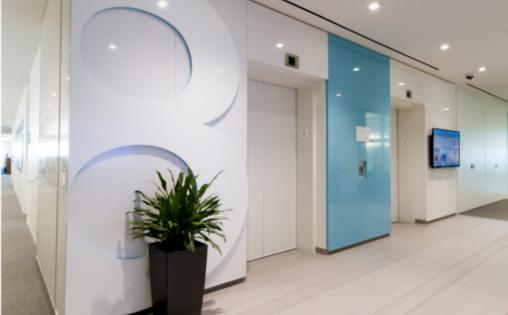
Lacquered glass is perfect for improving the aesthetics of your interiors due to its colour and light effects. The lacquer coating imparts brilliance to the glass and protects it from damage. It is also humidity-resistant and heat-resistant, and can be easily cut, drilled, ground and edge finished
